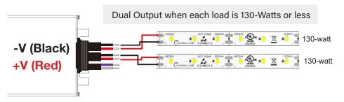
**NOTE:** If each output is OVER 130-Watts, combine outputs to 1 load by matching polarities (RED & RED) and (BLACK & BLACK).
